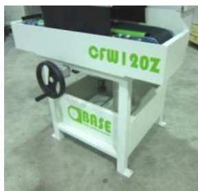
Water cooling system: integrated tank and pump
