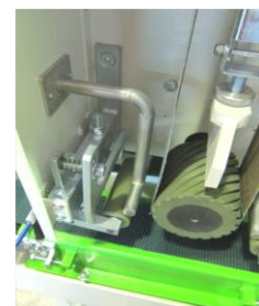
Contact roller with souble water spray
