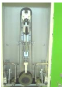
Abrasive belt head. Easy belt replacement: no tools needed
